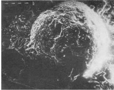
Fig. 10. Fractograph (16.9 \times ) of a PS-mortar composite prepared by 6 days ( \sim 15 Mrad) of irradiation. The picture shows a hollow sphere of polystyrene with a big perforation at lower right of the sphere. Some small perforations are also visible. Surface of the sphere is rough. Possibly, this is caused by an easy deformability of the polymer shell because of lower thickness, and does not indicate a stronger PS-mortar interfacial interaction.
