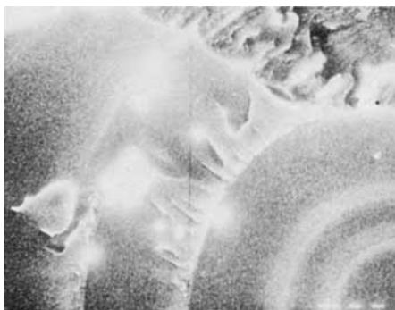
Fig. 9. An enlarged view (247 \times ) of Fig. 7 depicting several concentric beach marks with the divergent impression of the fracture waves propagating at right angles to the beach marks.
